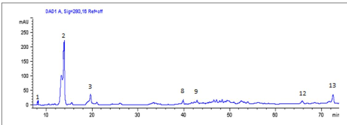
**Figure 5** - Phenolic profiles in the olives darkened by oxidation samples of Memecik variety.
