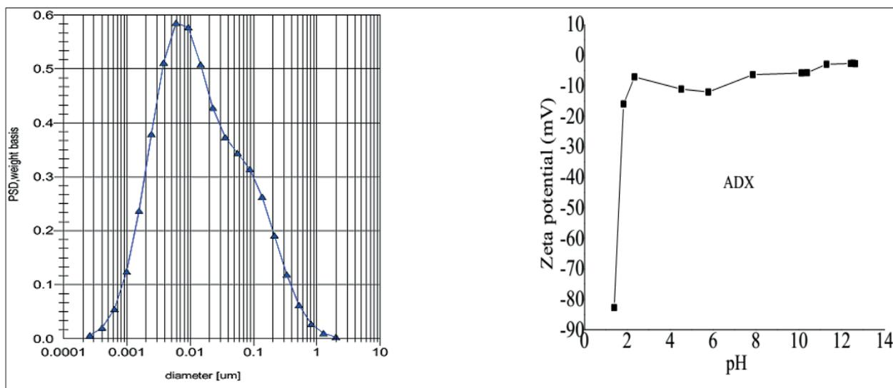
Figure 4 - PSD and zeta potential of ADX
