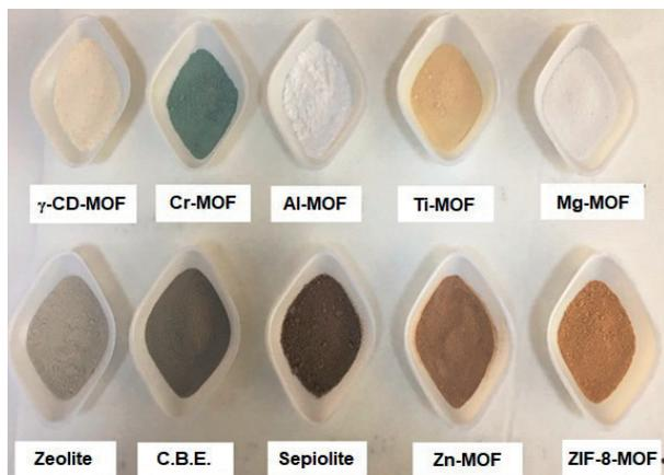
**Figure 1** - The MOFs and natural clays used as the adsorbent materials.
